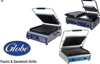
Stainless steel grills feature seasoned, cast iron griddle plates, machine-finished cooking surface, on/off switch, removable stainless steel catch tray, temperature range up to 570°F, and 3¹/2" adjustable feet. Panini grills have grooved plates; sandwich grills have smooth plates. NEW mid-size electric sandwich grill with combo plates - grooved top plate and smooth bottom plate GPGS1410. Models GPG14D, GSGDUE10, and GPGS1410 shown.
